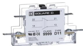
Contactor, Definite Purpose, auxiliary contact, 3A at 120 VAC, 1 NO contact and 1 NC contact, for 20A to 90A contactors
