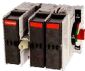
M25F12S 25A, NFC fused, 1 pole left of handle, 2 poles to the right, side operated
