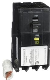
Mini circuit breaker, QO, 40A, 3 pole, 208Y/120VAC, 10kA, plug in, 6mA grd fault A, pigtail [TAA]
